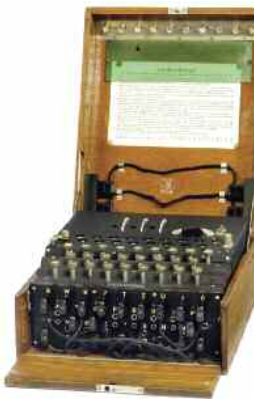
Enigma encoder machine used by the Germans during the World War II, to encode and decode war time messages
